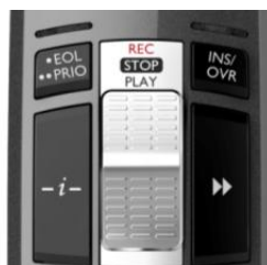
Slide switch operation (record, stop, play, rewind)
